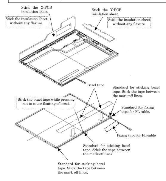
Figure 4-61 Replacing TMD fluorescent lamp (WXGA) (11)
